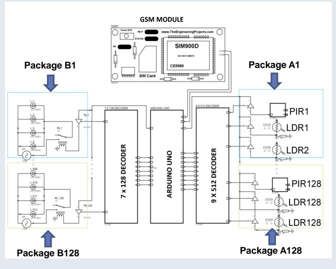
• GSM module is connected to the Arduino via RX, TX pins
